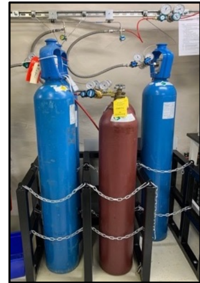
Gas cylinders (CO 2 , N 2 , O 2 ) are aged underground for a minimum of one month (N 2 source upgraded to LN 2 dewar in 2019)
